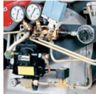
Example of the hydraulic circuit on RL70/M burners
