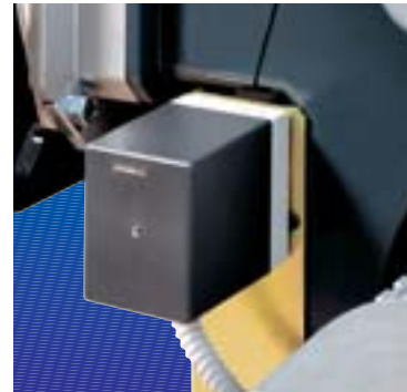
Example of the servomotor for air/oil setting
